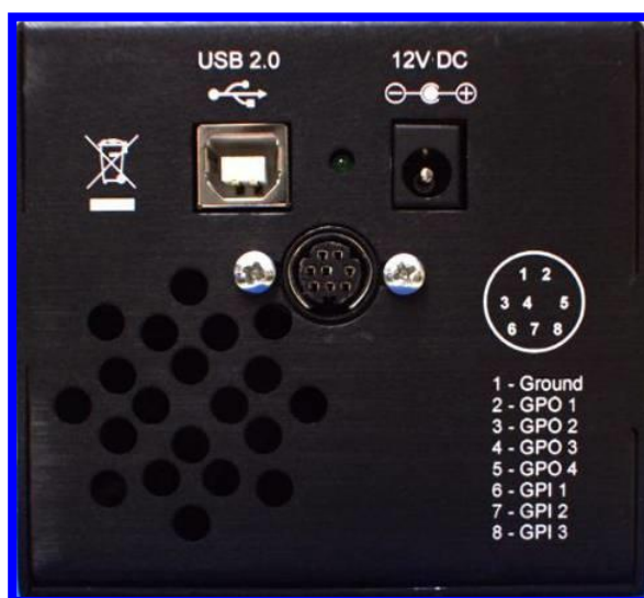
Figure 27: Large Format Camera External Header Location and Pin Numbering
