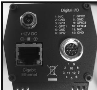
Figure 37: Lg Camera External Header Location and Pin Numbering
